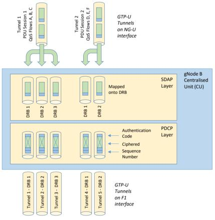
Figure 219 – SDAP and PDCP processing within the gNode B Centralised Unit (CU)
