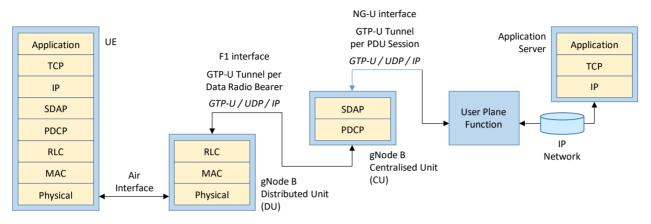
Figure 212 – User Plane protocol stack for Standalone Base Station
